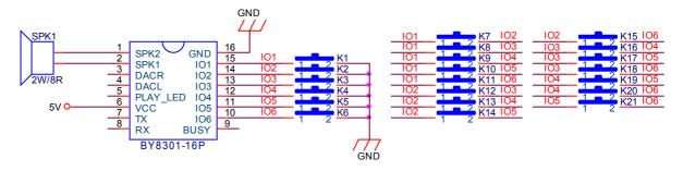
21-way switch button is equivalent to the amount of control.
