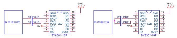
The module power is mainly the customer can own an external amplifier.
