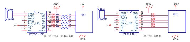
By the microcontroller through a low pulse signal (equivalent to pressing the lift button) can trigger IO1-IO6, achieve one Play six segments voice, and above 3IO selectable control modes.
