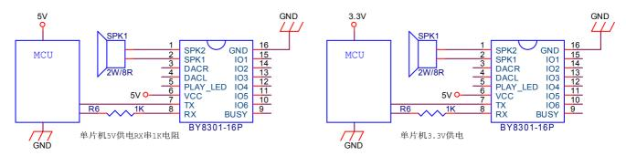
The above is a standard UART asynchronous serial connectivity applications, this application is quite flexible, including play, pause, up and down the song, volume addition and subtraction, Play selections, advertising spots and so on. Available microcontroller, computer serial port control 485 can also be controlled by TTL to RS485 adapter plate.
