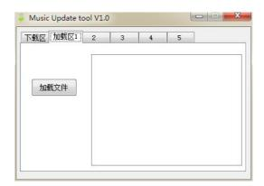
10.3. At this point you need to load the selected voice, you need to put on a one-time multi-stage election finished, the entire sequence can be selected into a loading area (area 2-5 are reserved function without load), and then click "Open" to add the software in the. Voice document proposes naming 0001XXX.mp3,0002XXX.mp3
